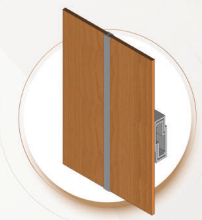
Undercut concealed fixation with joint connector
